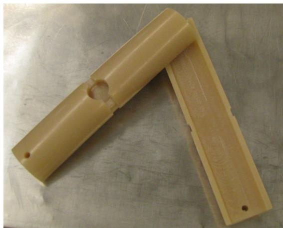
**FIGURE 1:** Polyethylene sample holder used in the dry tube irradiation
